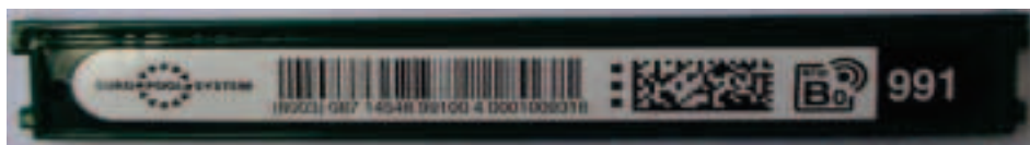
Figure 4.2-1: Identification ‘license plate’ RFID UHF for returnable packaging crates.
