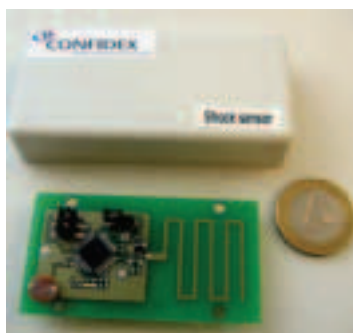
Figure 4.7-2: Prototype of a sensor-enabled tag, compatible with the EPC Gen2 protocol
