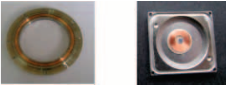
Figure 4.1-1: RFID tag embedded in the casing of a watch
